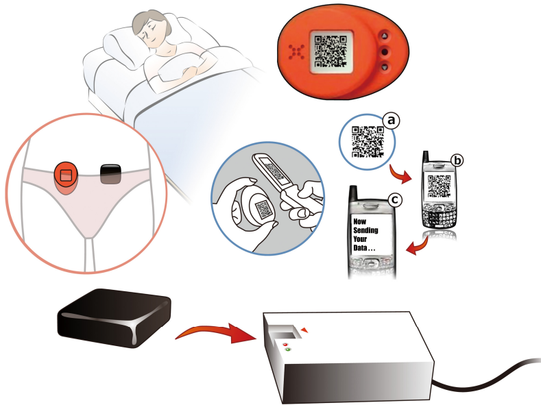
Fig. 10. A schematic drawing of the CBT and SBT data collection. Both the CBT and the SBT were measured automatically by clipping two wearable devices on a drawers strap on two sides of the subject's waist during sleep. The black cubic device was used for CBT data collection. The orange elliptic device was used to detect the SBT.
