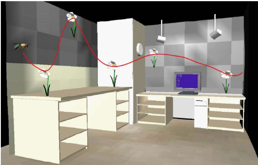
Fig. 2. The virtual reality environment for motor control learning; by generating adequate joint torque the subject can move the object (bee). The extension knee torque causes upward movement and the flexion torque a downward movement of the object, while the object moves in transversal plane synchronized (time) with the dynamometer.
