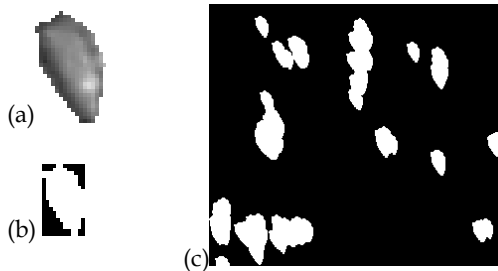
Fig. 6. Egg identification. (a) Average egg that was used to define (b) the structural element. (c) Image of Figure 5-right after application of the closing operator with the structural element of Figure 6-left-bottom.
